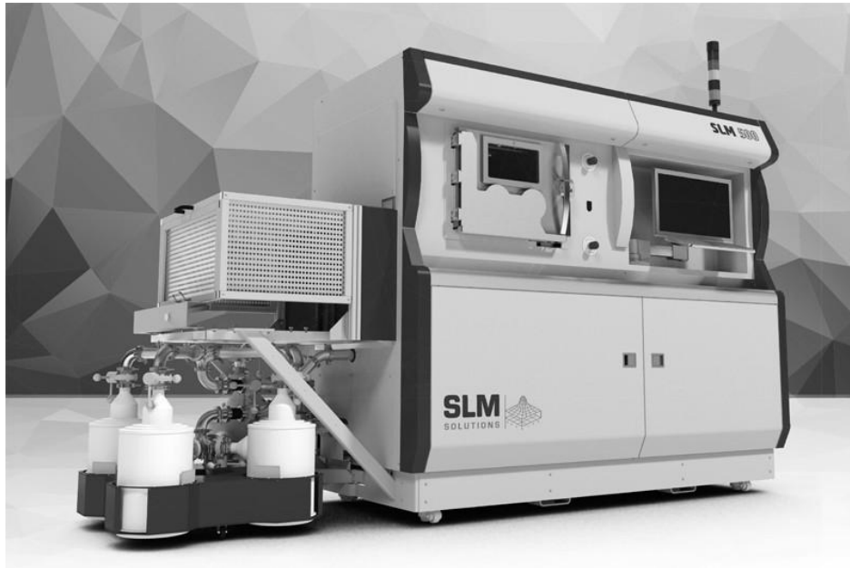
Fig. 11 – SLM machine with powder transport, sieving and storage occurring in a closed system with inert gas atmosphere. Source: SLM Solutions.
